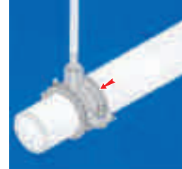
Fixing of Pipe with Clamp
